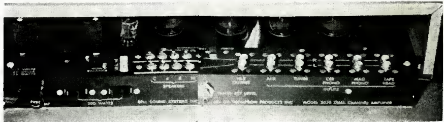
Above: rear view of amplifier showing inputs and outputs. The unit contains 11 tubes. Below: possible hookups for tape deck and amplifier plus associated equipment.
